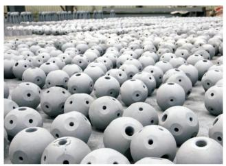
Connection ball with bolts hole for truss frame.
