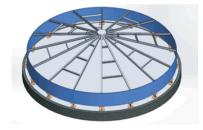
3. Install (assemble) and weld the truss of conic node
