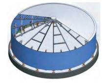
5. The electronic chain hoist pulls up , leading the tank rise, to rise the wallboard.
